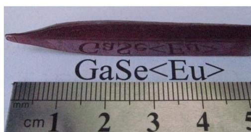
**Fig.1.** The image of *GaSe* single crystal doped with 0.025 at% *Eu*.
