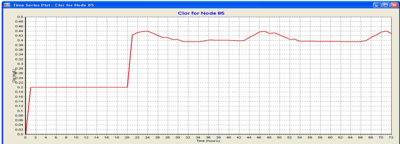
Fig.8. Variation of residual chlorine concentration in junction 85 after re-chlorination.
