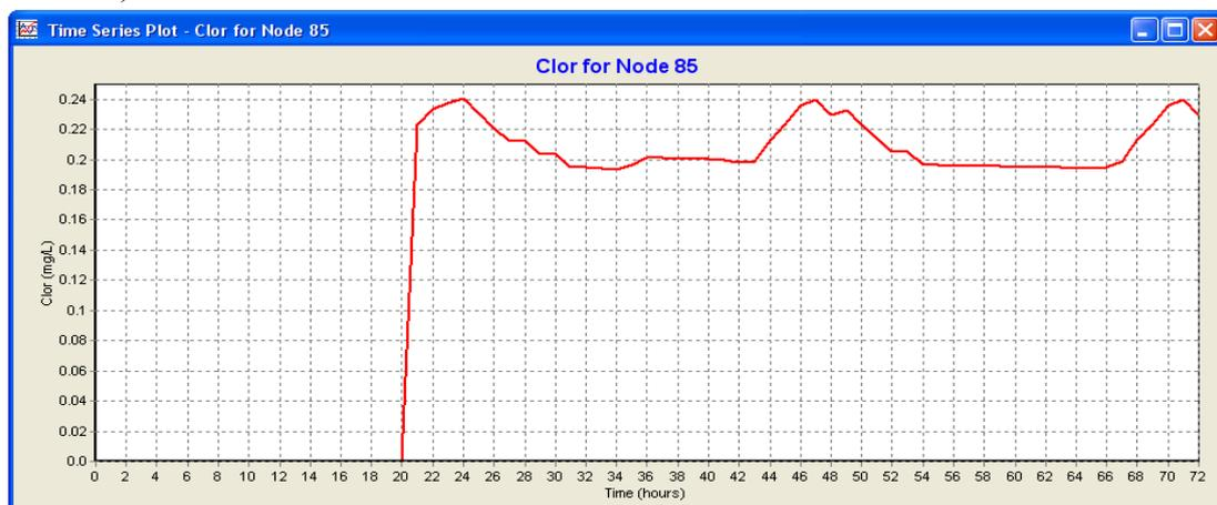
Fig.5. Residual chlorine concentration in junction 85 (Ohaba Strei).
