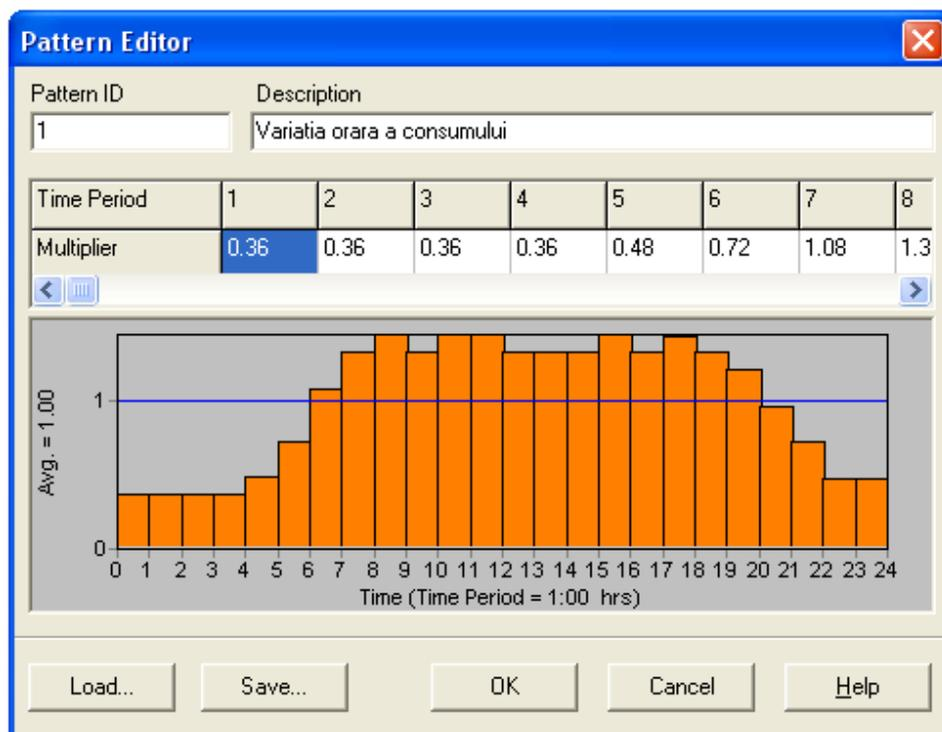
Fig.3. Hourly variation diagram for water consumption.
