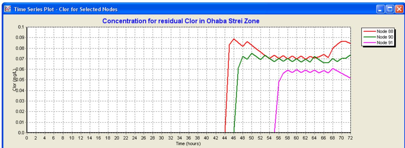
Fig.7. Variation of the residual chlorine concentration in Ohaba Strei area.
