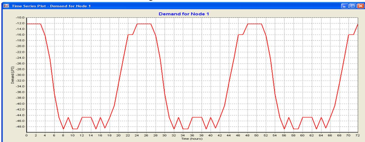
Fig.4. Water flow variation along the distribution network.
