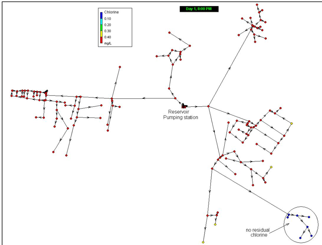
Fig.6. Residual chlorine concentration after 20 hours.
