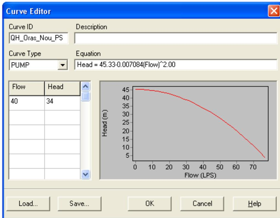
Fig.2. Pump's curve.
