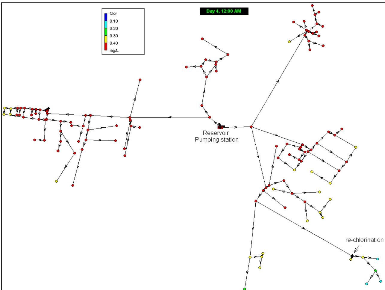
Fig.9. Variation of residual chlorine concentration in junction 85 after re-chlorination.
