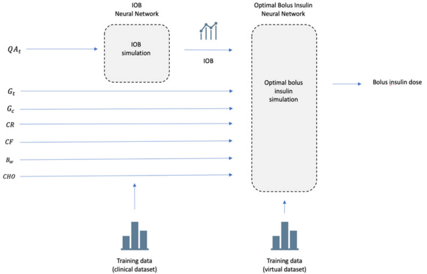
Fig. 1. Outline of the IOB and Optimal Bolus Insulin ANNs Structure of the Insulin-on-board (IOB) Neural Network.
